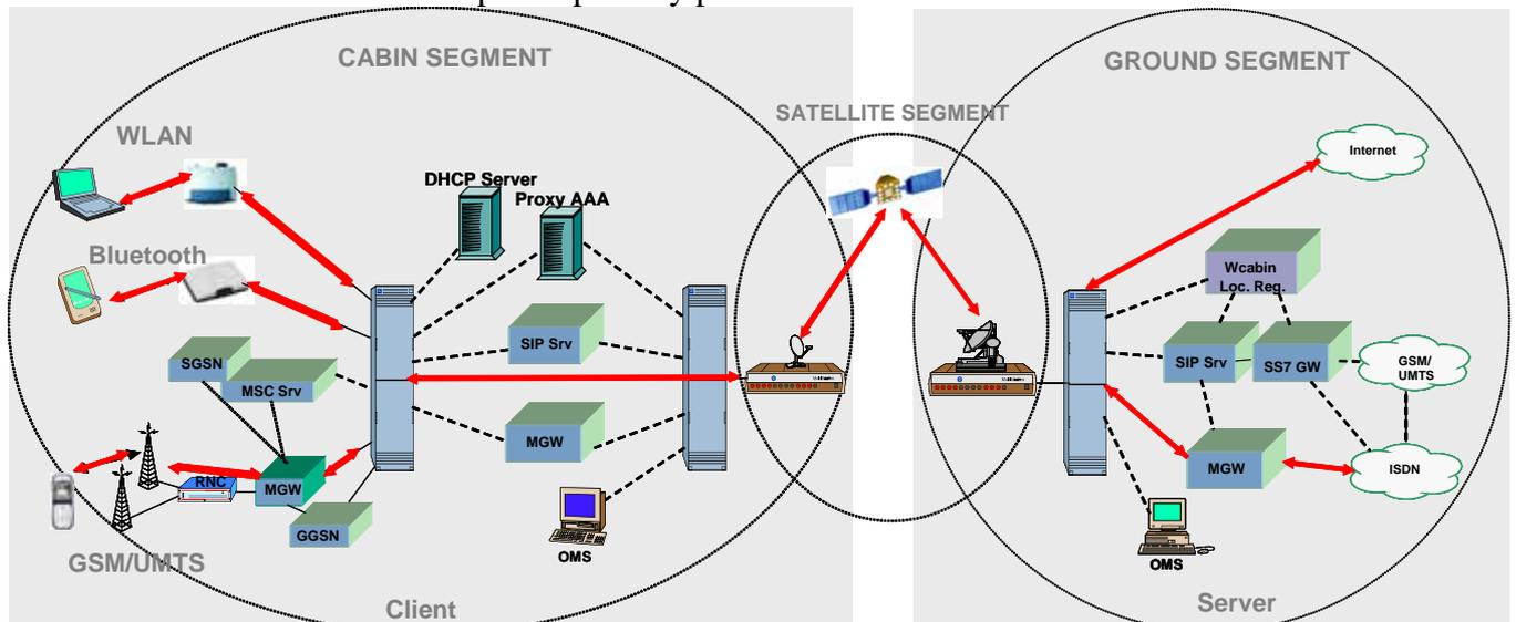
Fig 1 - Wireless Cabin System Architecture
